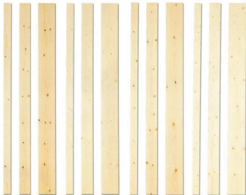
Grade G4-0 – Pine Grade A3 – Pine Grade III – Pine Grade G4-0 – Spruce Grade A3 – Spruce Grade III – Spruce Grade G4-1 – Pine Grade A4 – Pine Grade IV – Pine Grade G4-1 – Spruce Grade A4 – Spruce Grade IV – Spruce
